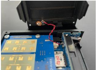
5. Unscrew the sensor holding screw.
