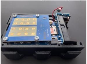
Use plastic stick to help it to go out - however be extremely careful to put only in the place shown in the figure and not putting it deeper than about 2 mm. There are electronic components on the bottom part that could be damaged. Go up to the point where you can hold the blue/white bord by the fingers and the continue using fingers.
