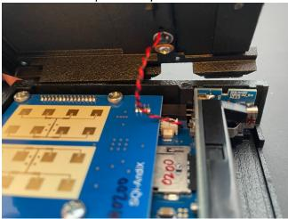
4. Gently turn the back of the case by 90 degrees while observing the black/red cable and not stressing it.
